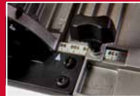
Double fence is anchored at the front and the back of the saw
