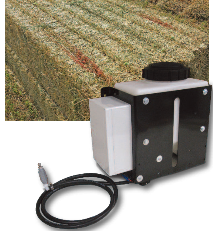
A hay bale marked when the alarm was set to 27%, showing the middle section is within the preferred moisture range, while the end flakes were above 27% moisture
