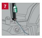
Install the pipe onto the valve and cut to the desired length.
