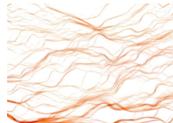
Fibrillation can be seen when the twine is untwisted. Good fibrillation gives good knotting properties.
